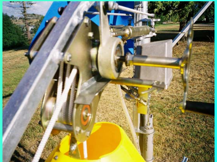
Cover removed to show rope capstan and governor
